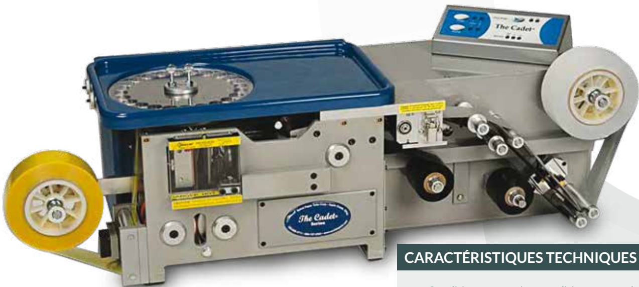
24002 - Cadet Vantage - 60 sachets/minute 24003 - Cadet Twin Vantage - 120 sachets/minute
